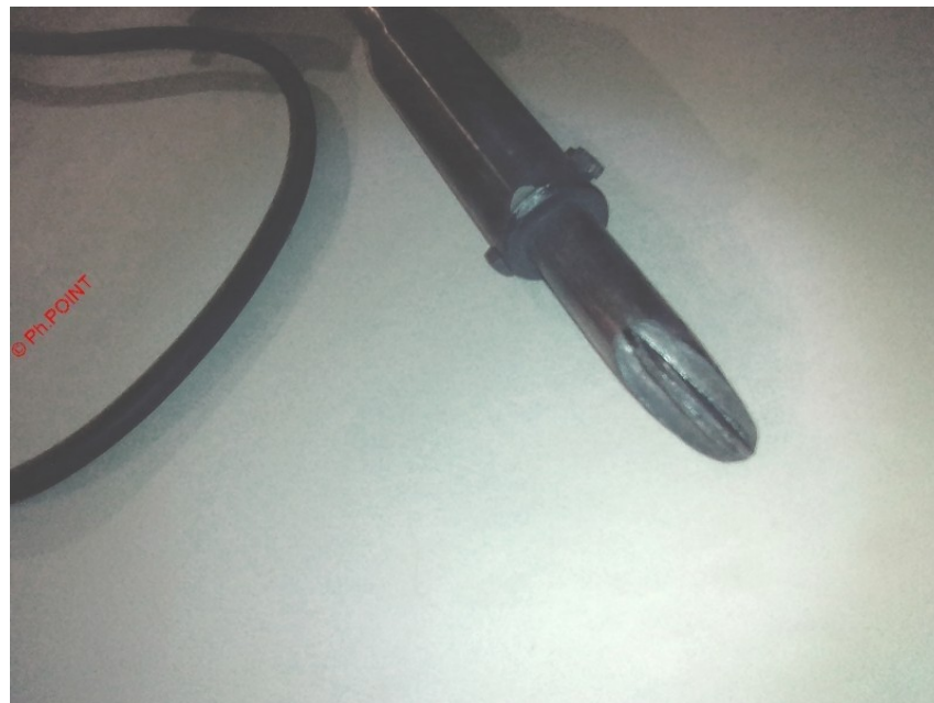
Illustration 49: Fabrication panne Cox [GSR_16]
